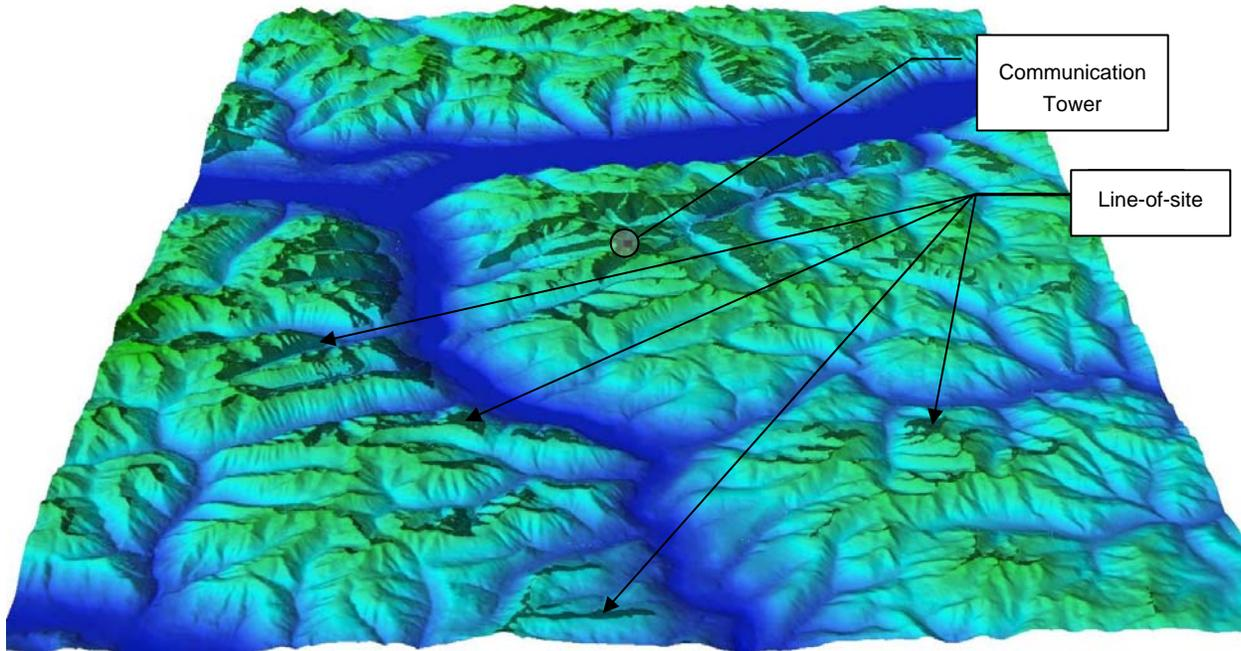
**Figure 4.** 3D Visualization of the LOS Examination for a sample map sheet for the Nelson, BC area. Dark patches represent area's visible from a communication tower of 50m.
